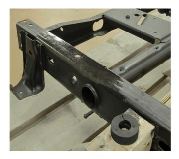
11. Apply a light flash-coat of Lloyds Kryptonite Metal Treatment P/N 36502 Life Long Rust Protection (14 ounce aerosol), or equivalent, to all rusted and bare areas of the frame where the wax coating was removed. This first coat should flash in approximately 3-5 minutes.
