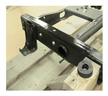
13. We suggest top coating the Lloyds Kryptonite with Daubert Nox-Rust® P/N X-121B "One Coat Rust Preventative Coating" (aerosol), or equivalent.
